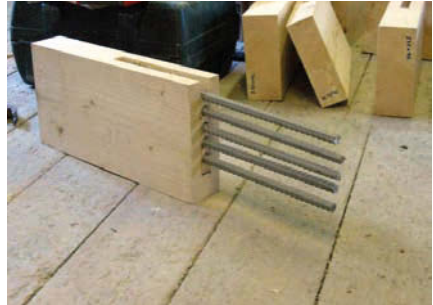
Fig. 4 New TRS ® with Stainless Rebar Rods
