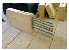
Fig. 4 New TRS® with Stainless Rebar Rods
